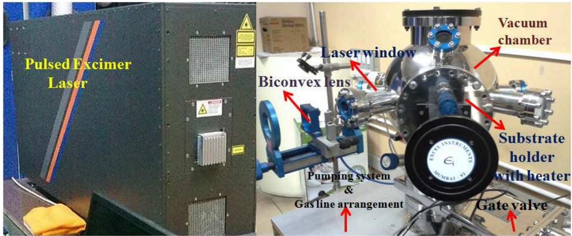
**Figure 2.4** PLD set up in our lab.
